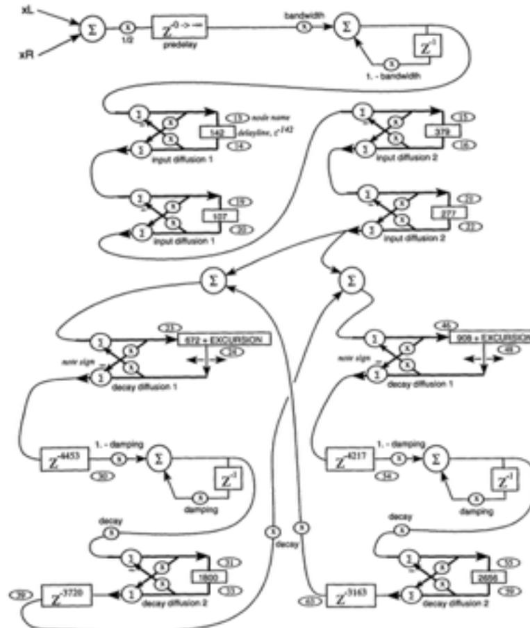
Fig. 1. Simplified plate-class reverberation topology in the style of Griesinger. For output tap structure ( $y_1$ ,  $y_2$ ) see Table 2. Delay-line taps at nodes 24 and 48 are modulating.
